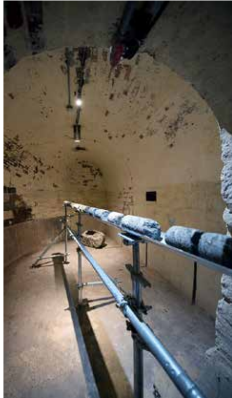
Detail of geologic core path entering the North Powder Magazine with sections of Manhattan schist and fossilized marine organisms visible.
